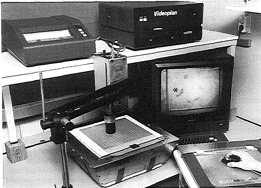
FIGURE 7. Equipment for enlargement of low-power micrographs connected to a semiautomatic image analysis system (Videoplan, Kontron Messgeräte, Eching, FRG). The micrographs on the illuminated screen are covered with an appropriate square lattice. One square is magnified with a video camera and the image is projected on the screen of the monitor. The black lines on the screen of the monitor correspond to the edges of the square of the lattice; the white lines delineate the "active area" of the Videoplan. *, Enlarged transversely cut synaptic contact zone after E-PTA treatment.
