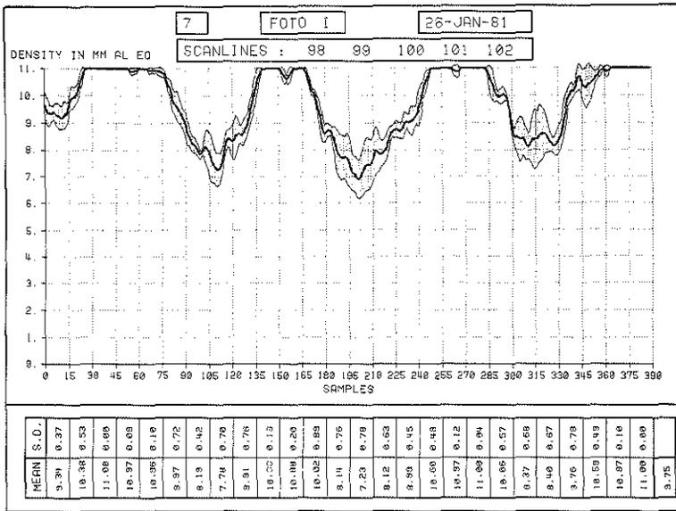
Fig. 25. Example of the spread of five horizontal trajectories of 0.2 mm and the average value (mean) in one radiograph. The mean Al. eq value over a scan length of one mm (15 samples) and the standard deviation of the five scans is given.
