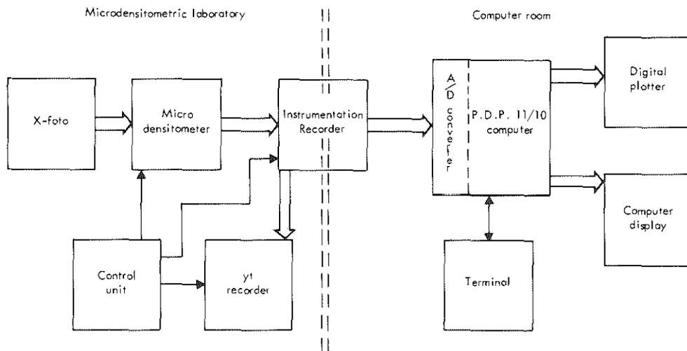
Fig. 9. Diagram of computing facility and microdensitometric laboratory.
