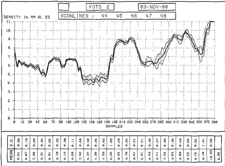
Fig. 10a, 10b. Radiograph and computer-generated scan showing the average Al. eq values/mm<sup>2</sup> and the standard deviation.
