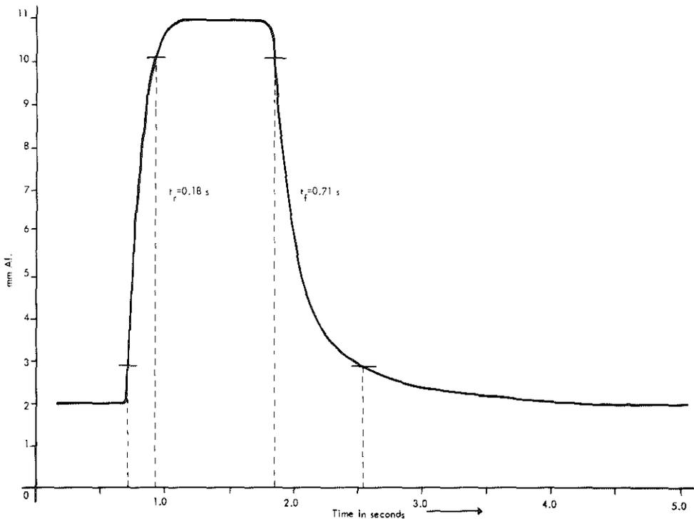
Fig. 20. Step-up and step-down response. The values indicated correspond to 10% and 90% of the total step height.
