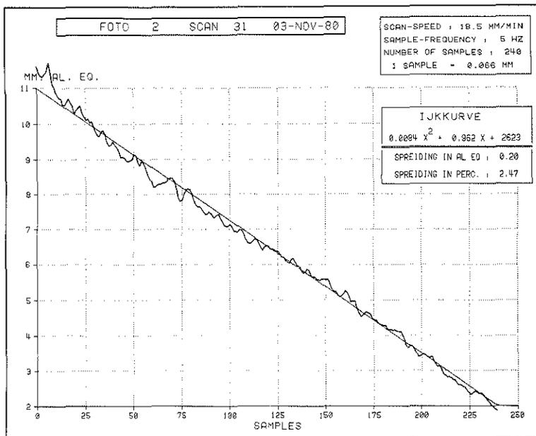
Fig. 3. The quadratic curve-fit shows the AL. eq values (11 - 2 mm AL) the straight line indicates the real AL. eq values, the curved line shows the AL. eq values of the wedge as computed according to the quadratic formula from the registered data.
