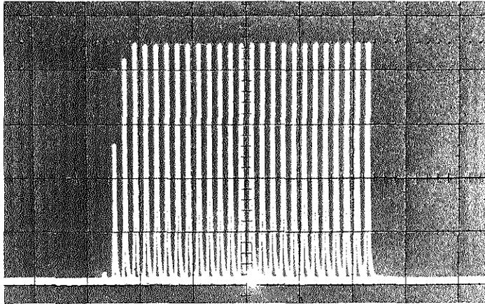
Fig. 13. Photograph of the monitor screen of the storage oscilloscope showing differences in output per each period of 1/50 sec. The oscillogram represents a set of radiation pulses. Especially during the initial stage, there is a reduction in the height of the pulses.
