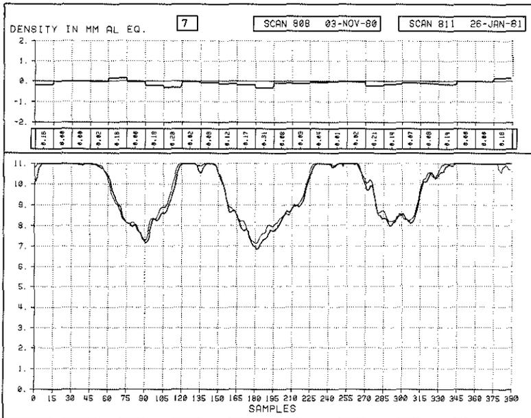
Fig. 26. The mean values, each representing the mean of 5 scans on 2 radiographs used to analyse the precision between exposures taken during one session.
