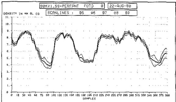
Fig. 16. Mean Al. eq value of the five scans and the standard deviation are shown. A one mm section of the curve track (sample 180 to 195) is evaluated in table IX.
