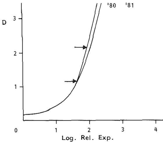
Fig. 15. Characteristic Curve Kodak Morelight U. Speed DF. 57. Standardised Processing. Investigation 1980 - 1981.
