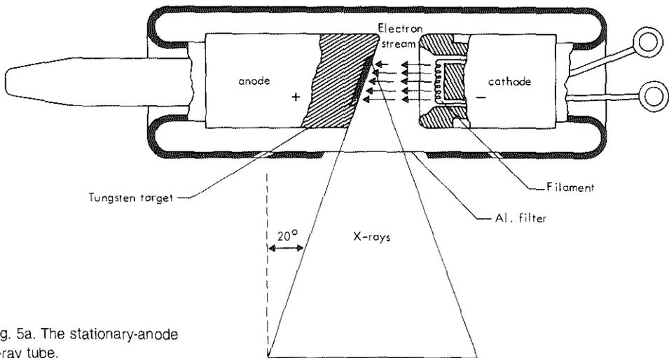
Fig. 5a. The stationary-anode X-ray tube.
