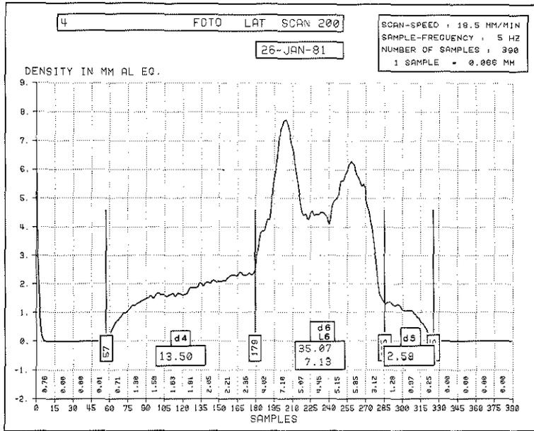
Fig. 31b. Illustrative scan in the centre of the middle phalanx Dig. II. of a lateral radiograph with soft tissue density values.  $d_4$  and  $d_5$ .
