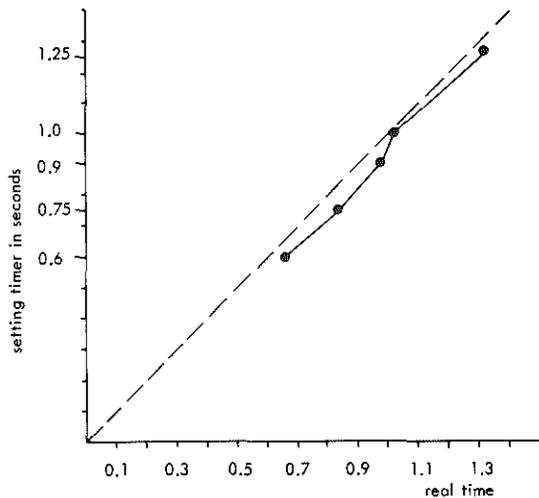
Fig. 14. Graph showing the relation between the exposure time and the exposure setting.
