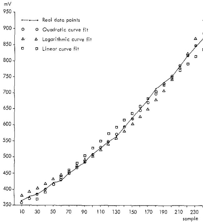
Fig. 1. Graph showing the output of the photomultiplier against the thickness of the wedge, the samples 10 to 230 were taken along the wedge (respectively from 11 - 2 mm Al.). The three mathematical curves are shown with three different symbols.
