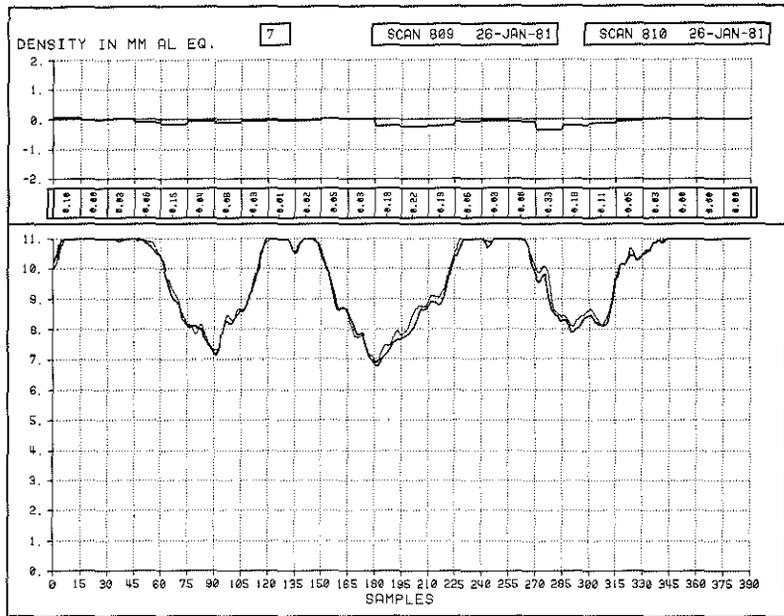
Fig. 27. Example of two scans illustrating the mean Al. eq values of two radiographs made during different sessions (interval of three months).
