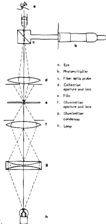
Fig. 6. Schematic drawing of a microdensitometer.
