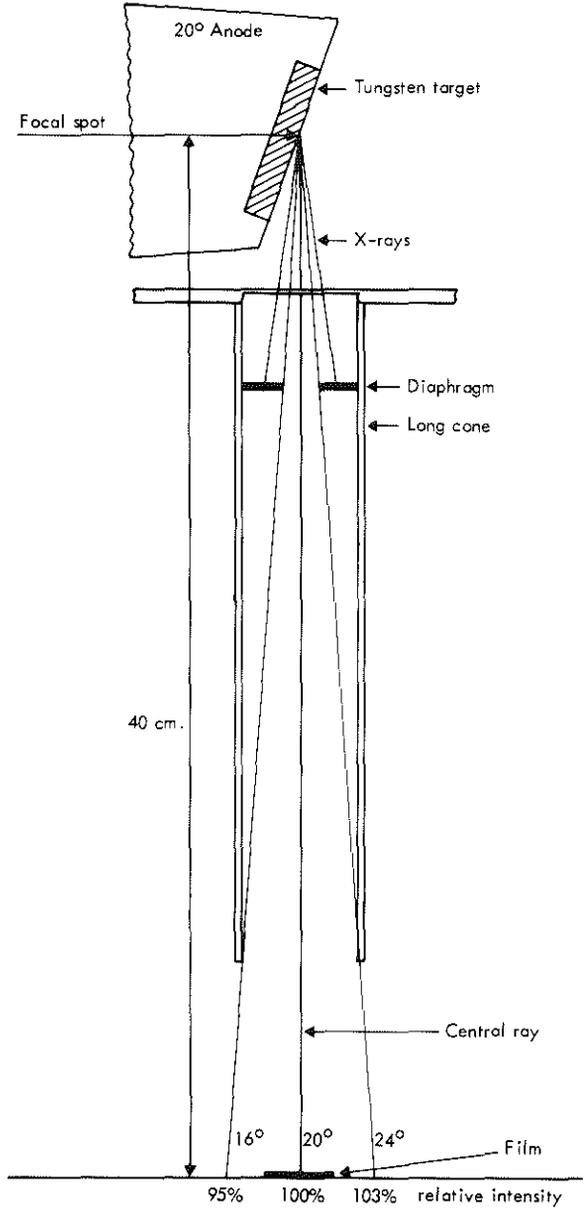
Fig. 5b. The heel-effect as given in the literature adapted to the long-cone technique (ref. The Fundamentals of Radiography).
